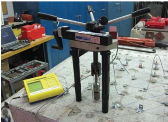
Research laboratory testing of powder-actuated ceiling hangers
