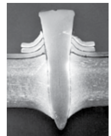
Figure 2: Robust anchorage - power-actuated fastener in steel.
